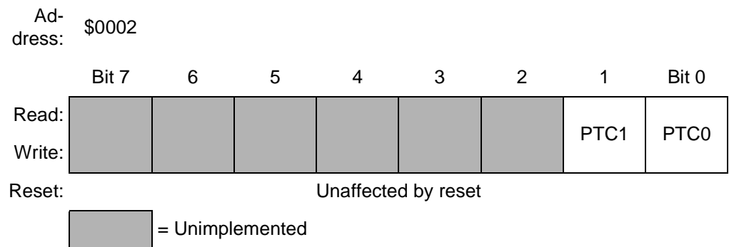
Figure 14-8. Port C Data Register (PTC)
