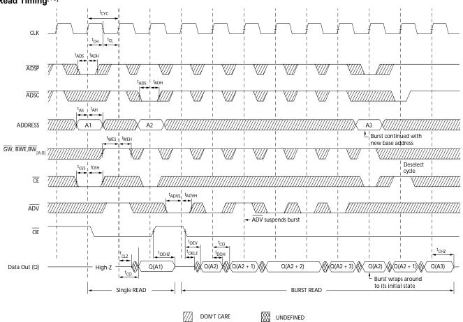
Note: 16. On this diagram, when  $\overline{CE}$  is LOW,  $\overline{CE}_1$  is LOW, CE2 is HIGH and  $\overline{CE}_3$  is LOW. When  $\overline{CE}$  is HIGH,  $\overline{CE}_1$  is HIGH or CE2 is LOW or  $\overline{CE}_3$  is HIGH.
