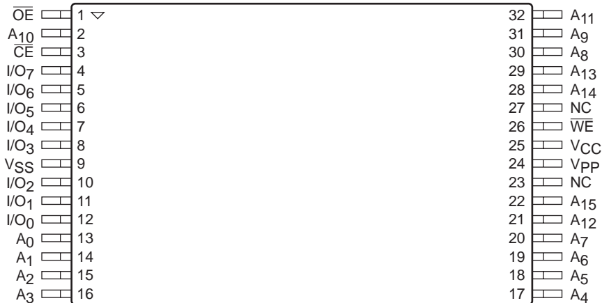
TSOP Package (Reverse Pinout) (TR)
