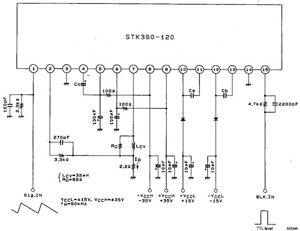
Notes. Ca, Cb (0 to 120pF) are for V<sub>CC</sub> switch noise suppression. Cc (47 to 220µF) is for supply switch ON shock noise suppression.
