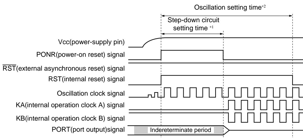
\* : 1:Step-down circuit setting time :  $2^{17}/\text{oscillation clock frequency}$  (oscillation clock frequency of 16 MHz: 8.19 ms)
