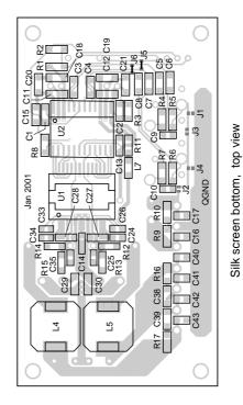
Fig.15 Printed-circuit board layout for TDA8926TH or TDA8927TH and TDA8929T.
