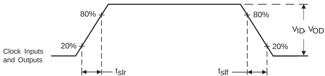
Figure 8. Input and Output Slew Rates
