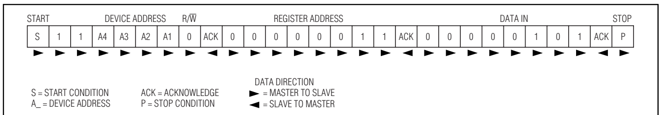
Figure 5. Example—Setting CLK3 to 80MHz
