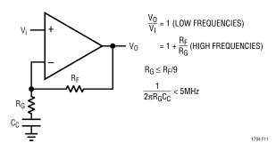
Figure 11. Alternate Noninverting Compensation
