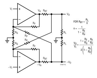
Figure 15. Back Termination Using Differential Postive Feedback
