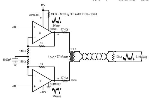
Figure 6. Estimating Line Driver Power Dissipation
