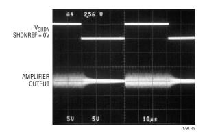
Figure 5. Shutdown and Recovery Timing
