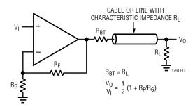
Figure 13. Standard Cable/Line Back Termination
