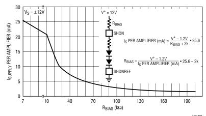
Figure 2. R<sub>BIAS</sub> to V<sup>+</sup> Current Control
