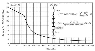
Figure 3. R<sub>BIAS</sub> to Ground Current Control
