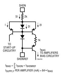
Figure 1. Internal Current Biasing Circuitry
