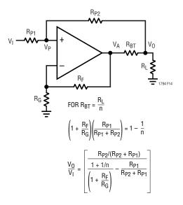
Figure 14. Back Termination Using Postive Feedback
