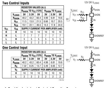
Figure 4. Providing Logic Input Control of Operating Current
