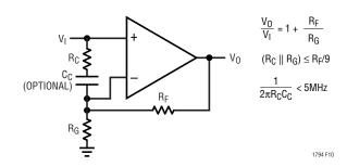
Figure 10. Compensation for Noninverting Gains
