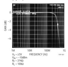
Closed-Loop Gain vs Frequency (A<sub>V</sub> = 2)
