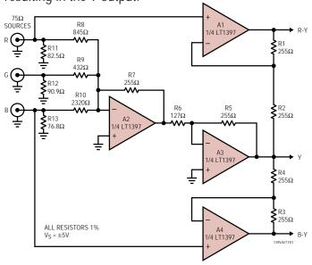
Figure 1. Buffered RGB to Color-Difference Matrix
