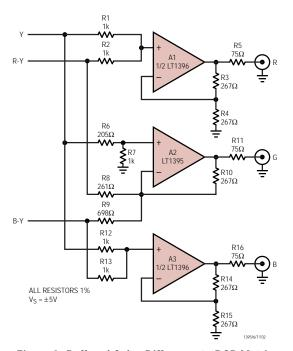
Figure 2. Buffered Color-Difference to RGB Matrix
