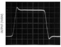
$V_S = \pm 5V$  $V_{IN} = \pm 2.5V$   $R_F = 374\Omega$  $R_L = 100\Omega$
