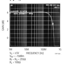
Closed-Loop Gain vs Frequency  $(A_V = -1)$
