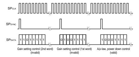
**Remark** Because gain setting control (2nd word) is input before gain setting control (1st word), gain setting control (1st word) becomes invalid. Then, because  $A/\mu$ -law, power down control is input even if gain setting control (1st word) is input, gain setting control (1st word) becomes invalid.
