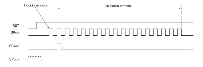
After ther RST pin has been set to the high level, input 1 clock or more to the SPclk pin, set the SPsyNc pin to the high level and input 16 clocks more to the SPclk pin.
