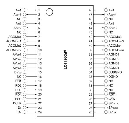
ACOMIN1-ACOMIN4 : Analog common voltage in Dx : Transmit PCM data out ACOMOUT1-ACOMOUT4: Analog common voltage out FSC : Frame synchronous clock in
