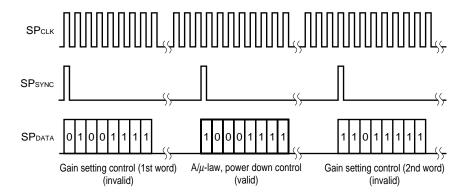
**Remark** Because A/ $\mu$ -law, power down control is input after input of gain setting control (1st word), gain setting control (1st word) becomes invalid and gain setting control (2nd word) also becomes invalid.
