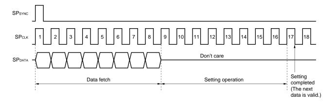
Ensure that 17 clocks or more are input to the SPclk pin between the rising of SPsyNc and the rising of the next SPsyNc.
