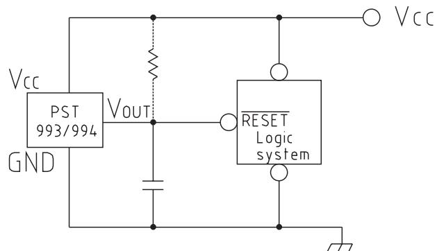
\* Since PST993 incorporates a constant current load, the pull-up resistance is not necessary.
