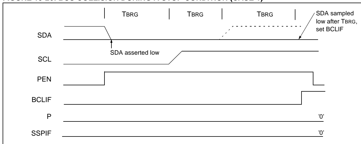
FIGURE 15-26: BUS COLLISION DURING A STOP CONDITION (CASE 1)
