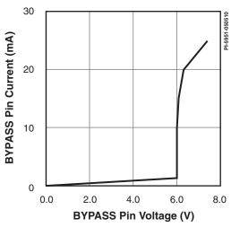
Figure 40. BYPASS Pin Current vs. BYPASS Pin Voltage.
