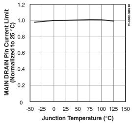
Figure 33. Main Supply. Internal Current Limit vs. Temperature.
