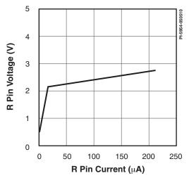
Figure 37. R Pin Voltage vs. R Pin Current.
