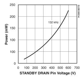
Figure 48. Standby Supply. Power vs. Drain Voltage.
