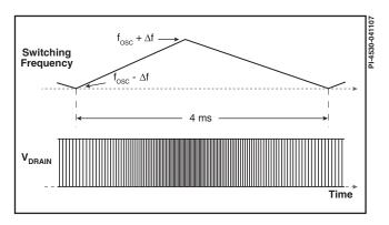
Figure 5. Switching Frequency Jitter (Idealized V<sub>DBAIN</sub> Waveforms).
