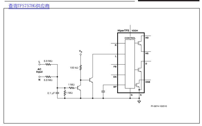
Figure 24. Fast AC Reset of BP Latch.
