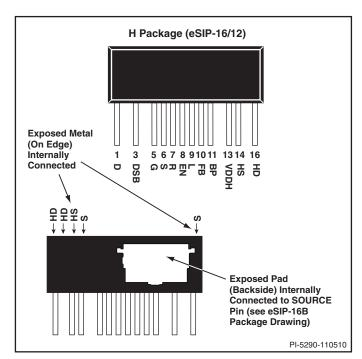
Figure 2. Pin Configuration.
