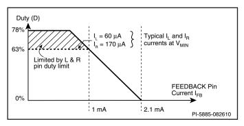
Figure 7. PWM Duty Cycle vs. Control Current.
