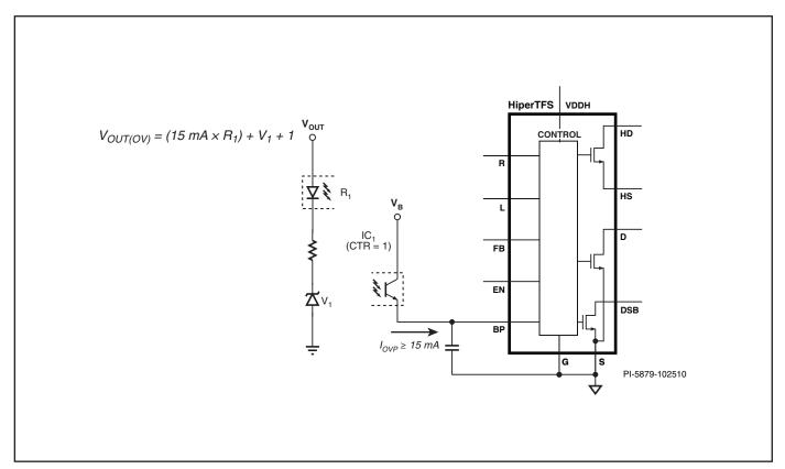
Figure 19. Latching Output OVP.
