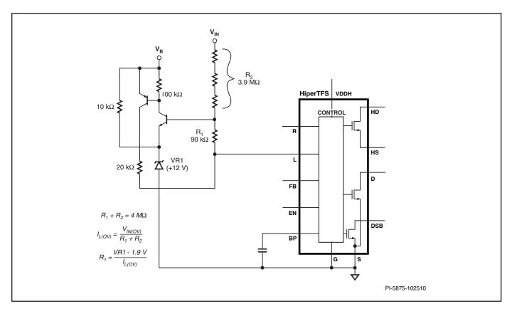
Figure 23. Non-latching Input OVP.
