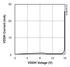
Figure 41. VDDH Current vs. VDDH Voltage.
