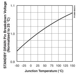
Figure 30. Standby Supply. Breakdown vs. Temperature.
