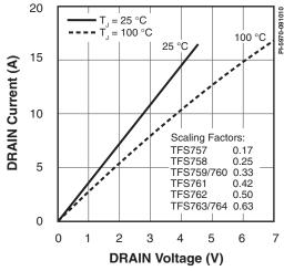
Figure 50. High-Side MOSFET Drain Current vs. Drain Voltage.
