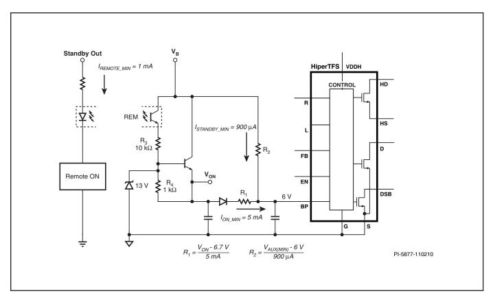
Figure 21. Remote ON and Standby Bias.
