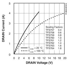
Figure 45. Drain Supply. Output Characteristics.
