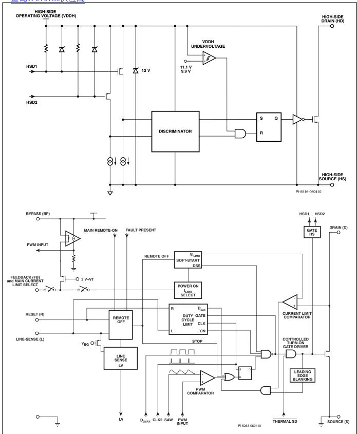
Figure 3. Functional Block Diagram for Two-Switch Forward Converter.
