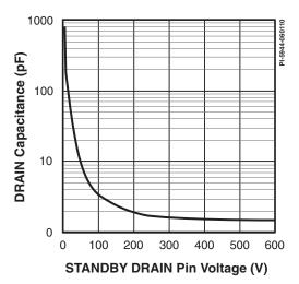
Figure 46. Standby Supply. Drain Capacitance vs. Drain Voltage.
