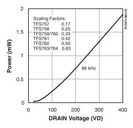
Figure 53. High-Side MOSFET Power vs. Drain Voltage.
