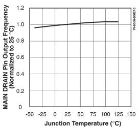
Figure 31. Main Supply. Frequency vs. Temperature.
