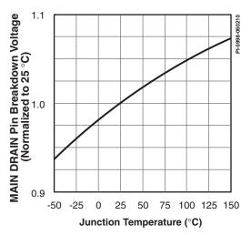
Figure 29. Main Supply. Breakdown Voltage vs. Temperature.
