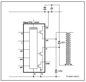
Figure 15. Typical Primary Winding Clamp-to-Rail.
