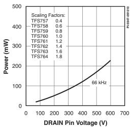
Figure 49. Main Supply. Power vs. Drain Voltage.
