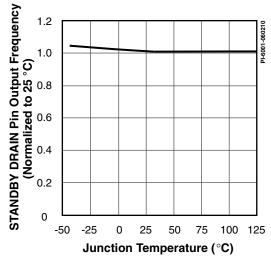
Figure 32. Standby Supply. Frequency vs. Temperature.
