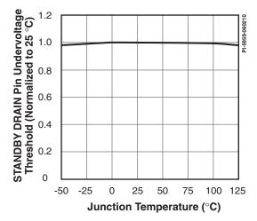
Figure 35. Standby Supply. Undervoltage Threshold vs. Junction Temperature.
