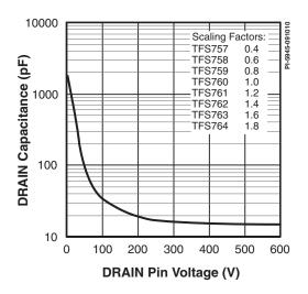
Figure 47. Main Supply. Drain Capacitance vs. Drain Voltage.
