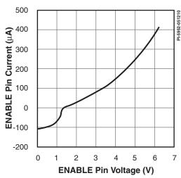
Figure 39. ENABLE Pin Current vs. ENABLE Pin Voltage.
