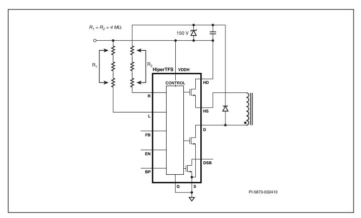
Figure 25. L and R Pin Reset and Duty Limit Circuit.
