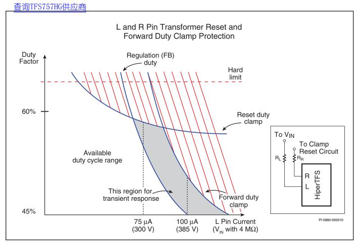
Figure 26. L and R Pin Duty Limit With  $R_1 = 4 M\Omega$  and  $R_B = 4 M\Omega$ .
