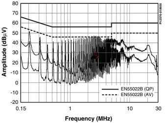
Figure 13. Fixed Frequency Operation Without Jitter.
