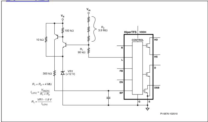
Figure 22. Input OVP (Latching).
