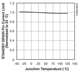
Figure 34. Standby Supply. External Current Limit vs.  $Temperature\ with\ R_{\shortparallel}=10.5\ k\Omega$
