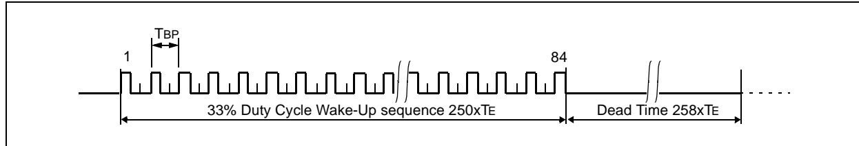
FIGURE 8-6: VPWM WAKE-UP FORMAT (MOD=1)
