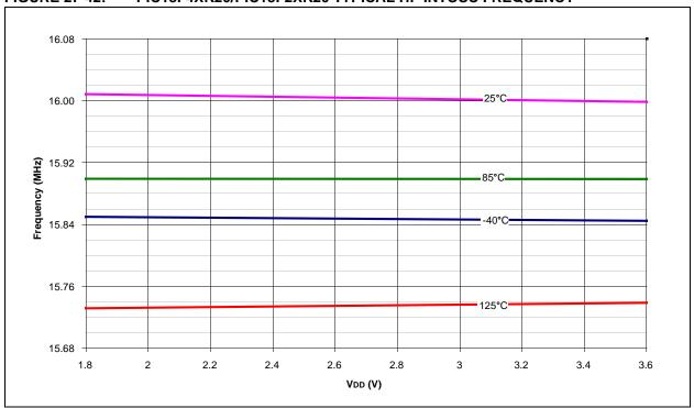
FIGURE 27-43: PIC18F4XK20/PIC18F2XK20 TYPICAL HF-INTOSC FREQUENCY
