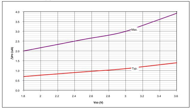
FIGURE 27-18: PIC18F4XK20/PIC18F2XK20 ∆IBOR and ∆IHLVD – Delta IPD for Brownout Reset and High/Low Voltage Detect, -40°C to +125°C
