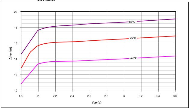
FIGURE 27-21: PIC18F4XK20/PIC18F2XK20 ∆locsB – Maximum Delta IPD for High Power Timer1 Oscillator
