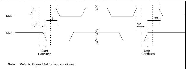
TABLE 26-20: MASTER SSP I<sup>2</sup>C™ BUS START/STOP BITS REQUIREMENTS
