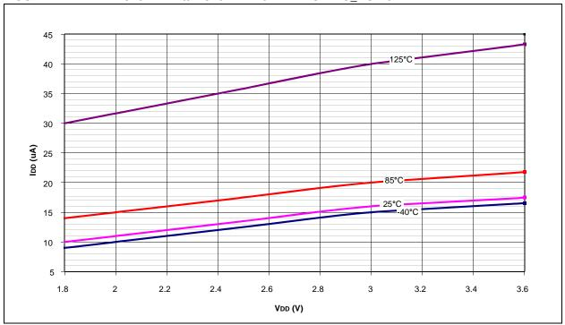
FIGURE 27-5: PIC18F4XK20/PIC18F2XK20 TYPICAL RC\_RUN IDD
