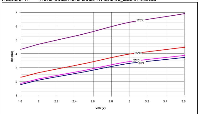
FIGURE 27-8: PIC18F4XK20/PIC18F2XK20 MAXIMUM RC\_IDLE 31 KHZ IDD
