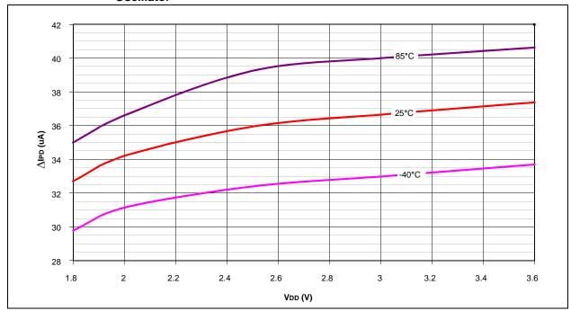
FIGURE 27-22: PIC18F4XK20/PIC18F2XK20 △ICVREF – Delta IPD for Comparator Voltage Reference, -40°C to +125°C
