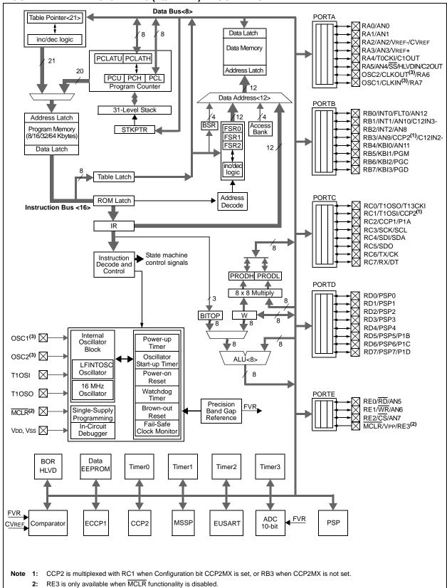
OSC1/CLKIN and OSC2/CLKOUT are only available in select oscillator modes and when these pins are not being used as digital I/O.
