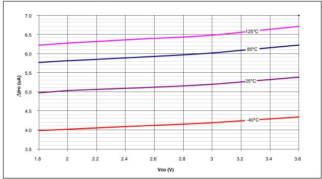
FIGURE 27-26: PIC18F4XK20/PIC18F2XK20 \( \text{\Discrete} \) Icomp - Maximum Delta IPD for Comparator in Low Power Mode, -40°C to +125°C
