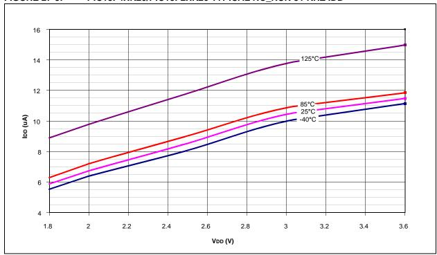
FIGURE 27-4: PIC18F4XK20/PIC18F2XK20 MAXIMUM RC\_RUN 31 KHZ IDD
