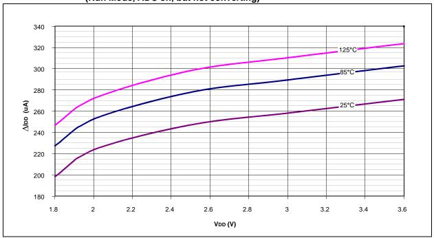
FIGURE 27-24: PIC18F4XK20/PIC18F2XK20 △IAD – Maximum Delta IDD for ADC, 25°C to +125°C (Run Mode, ADC on, but not converting)
