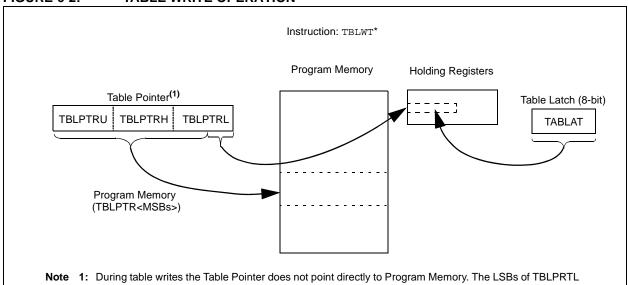
Note 1: During table writes the Table Pointer does not point directly to Program Memory. The LSBs of TBLPRTL actually point to an address within the write block holding registers. The MSBs of the Table Pointer determine where the write block will eventually be written. The process for writing the holding registers to the program memory array is discussed in Section 6.5 "Writing to Flash Program Memory".
