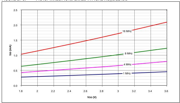
FIGURE 27-10: PIC18F4XK20/PIC18F2XK20 MAXIMUM RC\_IDLE IDD
