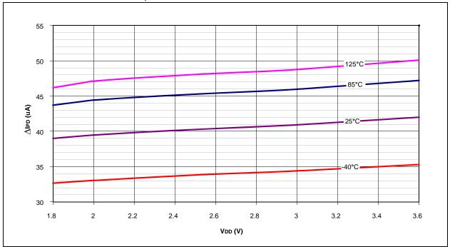
FIGURE 27-28: PIC18F4XK20/PIC18F2XK20 △ICOMP – Maximum Delta IPD for Comparator in High Power Mode, -40°C to +125°C
