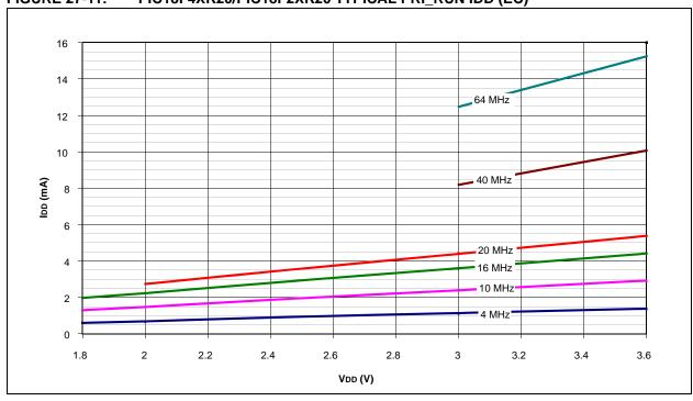
FIGURE 27-12: PIC18F4XK20/PIC18F2XK20 MAXIMUM PRI\_RUN IDD (EC)
