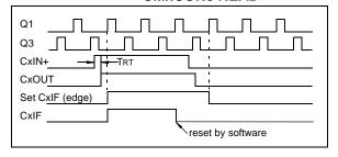
FIGURE 20-5: COMPARATOR INTERRUPT TIMING WITH CMxCON0 READ
