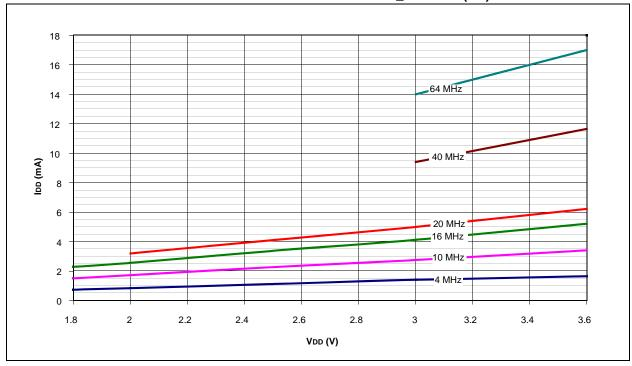
FIGURE 27-13: PIC18F4XK20/PIC18F2XK20 TYPICAL PRI\_RUN IDD (HS + PLL)
