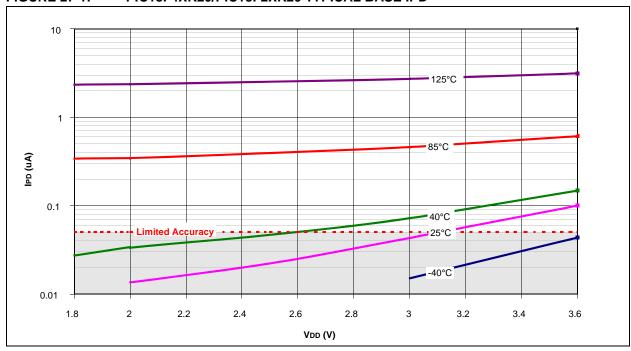
FIGURE 27-2: PIC184XK20/PIC18F2XK20 MAXIMUM BASE IPD
