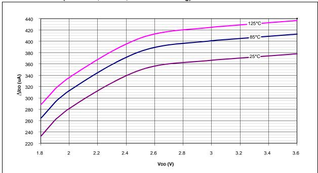
FIGURE 27-25: PIC18F4XK20/PIC18F2XK20 \( \text{\DeltaIcomp} - Typical Delta IPD for Comparator in Low Power Mode, -40°C to +125°C
