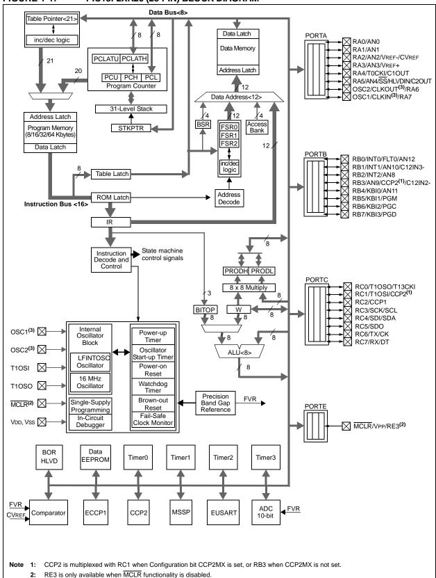
OSC1/CLKIN and OSC2/CLKOUT are only available in select oscillator modes and when these pins are not being used as digital I/O.
