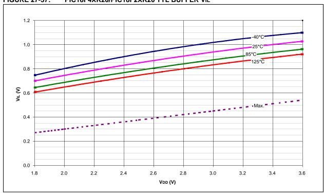
FIGURE 27-38: PIC18F4XK20/PIC18F2XK20 SCHMITT TRIGGER BUFFER VIL
