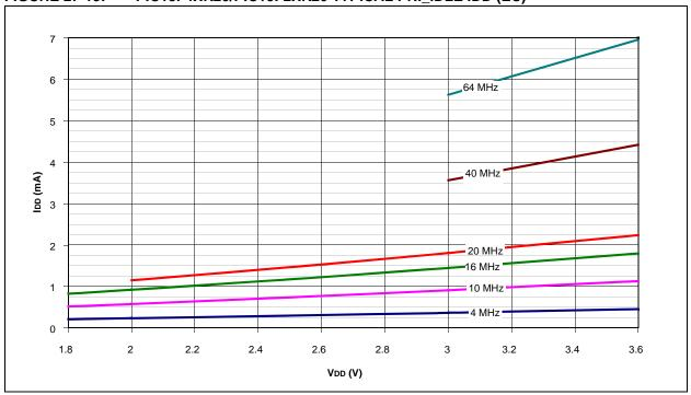
FIGURE 27-16: PIC18F4XK20/PIC18F2XK20 MAXIMUM PRI\_IDLE IDD (EC)
