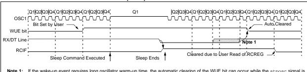
Note 1: If the wake-up event requires long oscillator warm-up time, the automatic clearing of the WUE bit can occur while the stposc signal is still active. This sequence should not depend on the presence of Q clocks.
