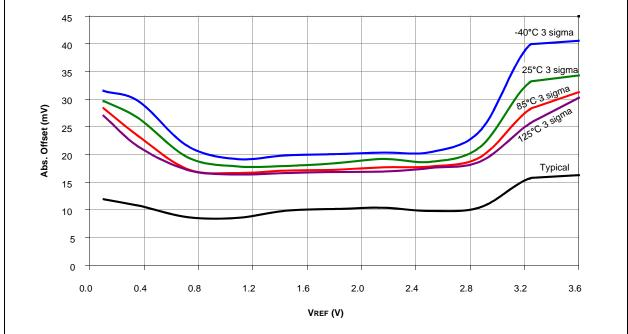
FIGURE 27-33: PIC18F4XK20/PIC18F2XK20 TYPICAL FIXED VOLTAGE REFERENCE
