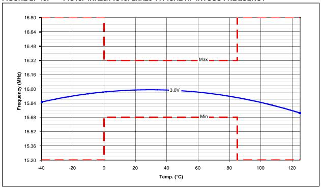
FIGURE 27-44: PIC18F4XK20/PIC18F2XK20 TYPICAL LF-INTOSC FREQUENCY (MAX./MIN. = 31.25 KHZ +/-15%)
