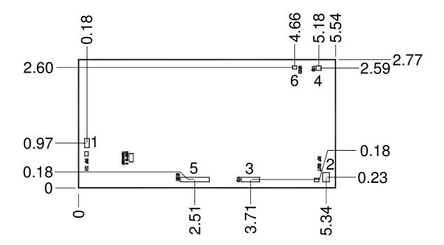
Units: millimeters Thickness: 0.10 Die x,y size tolerance: +/- 0.050 Chip edge to bond pad dimensions are shown to center of pad Ground is backside of die
