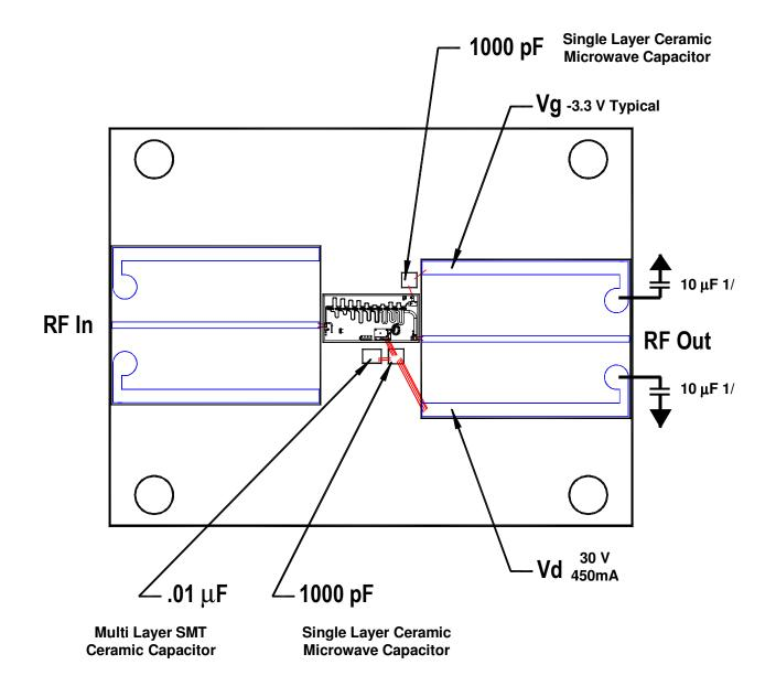
1/ Additional bypass capacitors may be required at this location. The presence and value of these capacitors varies by application. Variables include power supply impedance, power supply stability with reactive loads, and the inductance from the power supply to this assembly. 1 to 47 uF tantalum capacitors are commonly used here.
