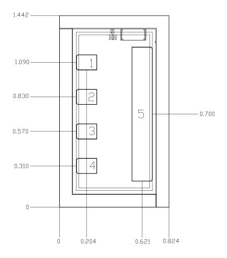
Units: millimeters Thickness: 0.100 Die x,y size tolerance: +/- 0.050 Chip edge to bond pad dimensions are shown to center of pad Ground is backside of die
