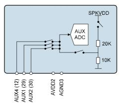
Figure 24 Auxiliary ADC Inputs
