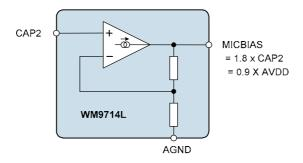
Figure 22 Microphone Bias Schematic
