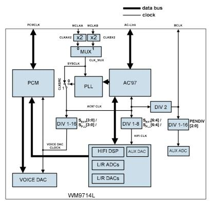
Figure 10 Clocking Architecture for WM9714L
