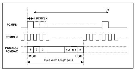
Figure 14 PCM Interface Mono Mode (mode B, FSP=1)
