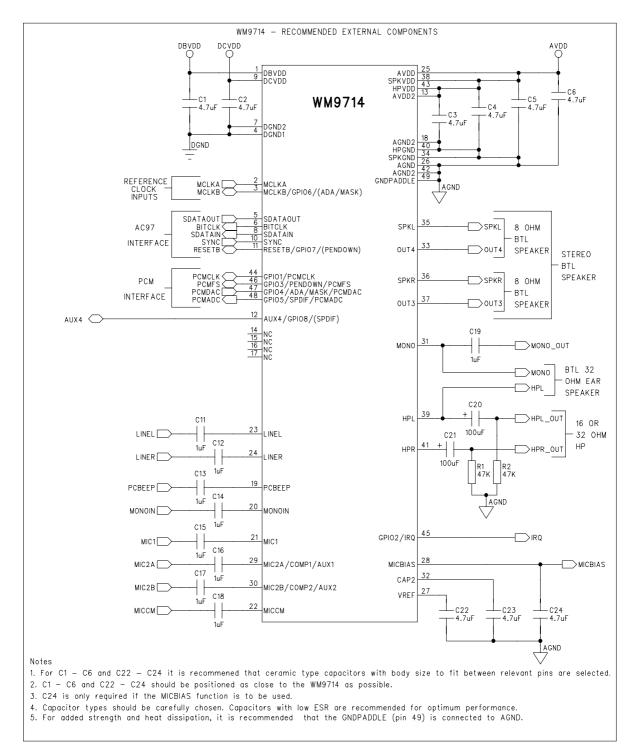
Figure 28 Recommended External Component Diagram
