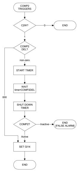
Figure 26 COMP2 Delay Flow Chart
