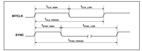
Figure 1 Clock Specifications (50pF External Load)
