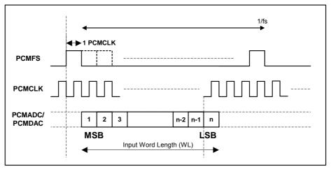
Figure 13 PCM Interface Mono Mode (mode A, FSP=0)
