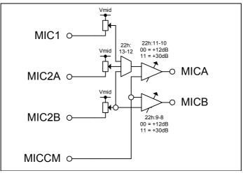
Figure 20 Microphone Input Circuit
