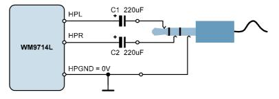
Figure 30 Simple Headphone Output Circuit Diagram
