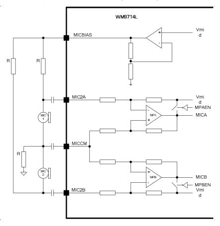
Figure 21 Dual Microphone Configuration
