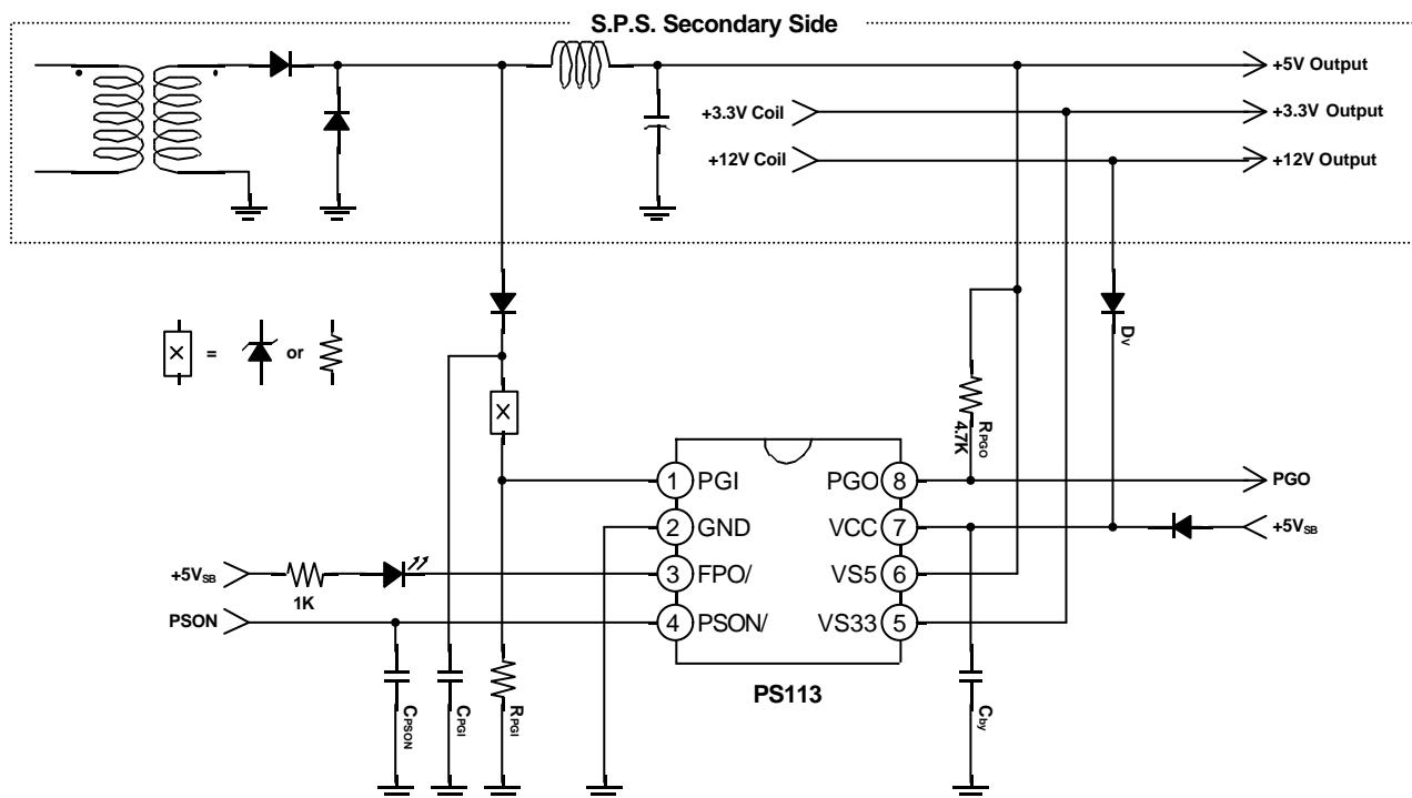
Note1: Zener diode or resistor or both of them can be used in component X.
