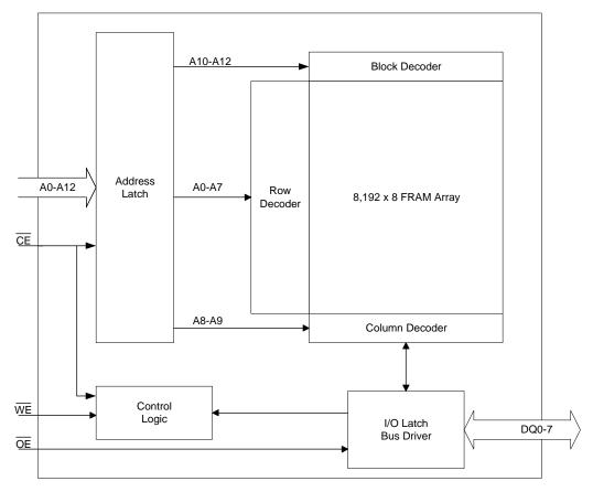
Figure 1. Block Diagram
