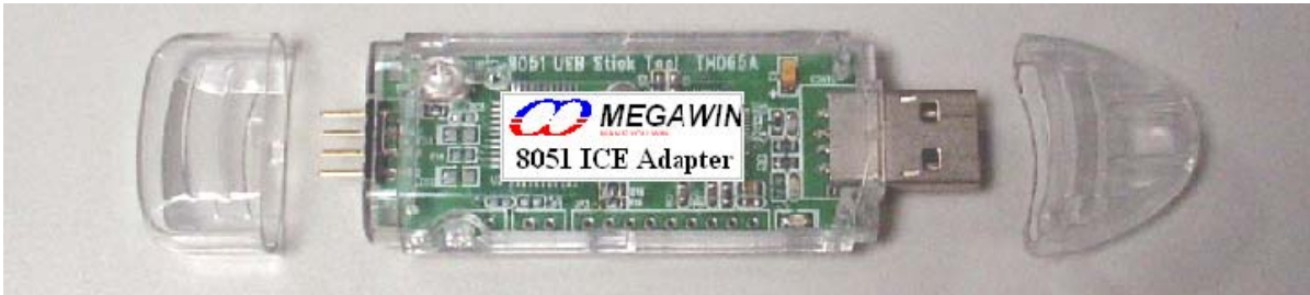
Figure 28-2. System Diagram for the ICE Function
