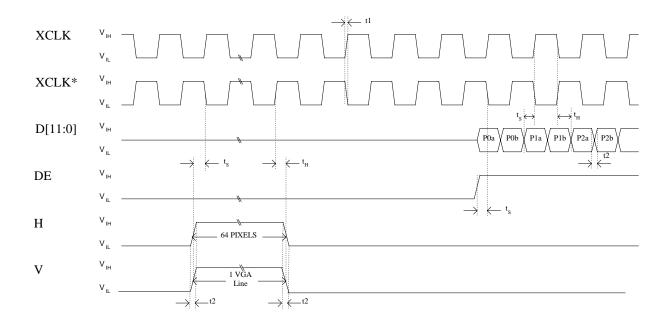
Figure 6: Timing for Clock - Slave, Sync - Slave Mode
