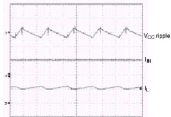
Figure 25. Boost Input Voltage and Current Ripple Waveforms
