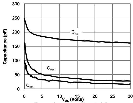
**Figure 8: Capacitance Characteristics**
