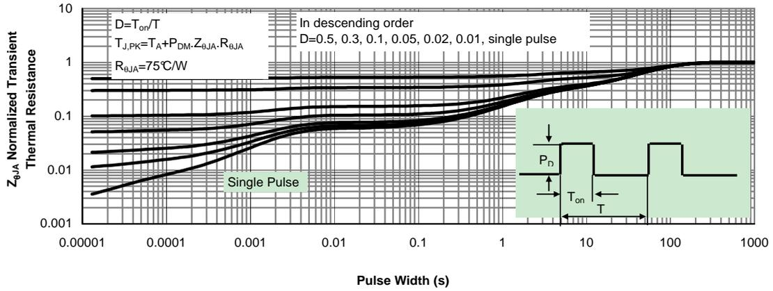
Figure 12: Normalized Maximum Transient Thermal Impedance (Note F)
