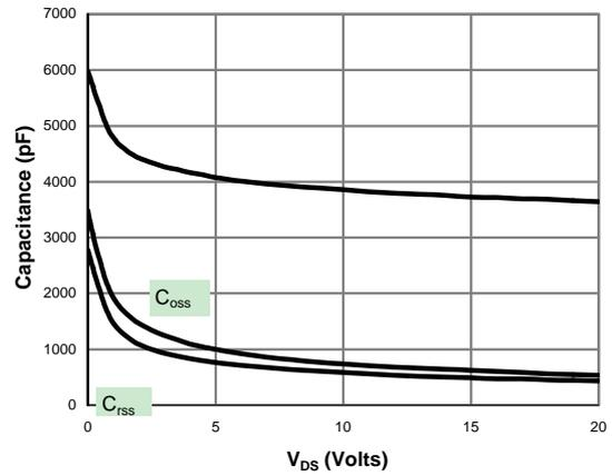
Figure 8: Capacitance Characteristics
