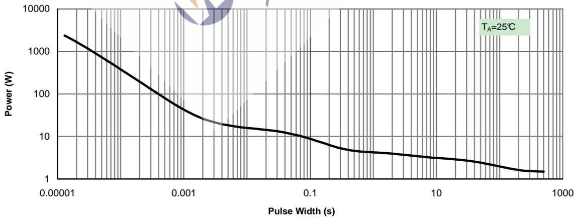
Figure 11: Single Pulse Power Rating Junction-to-Ambient (Note F)
