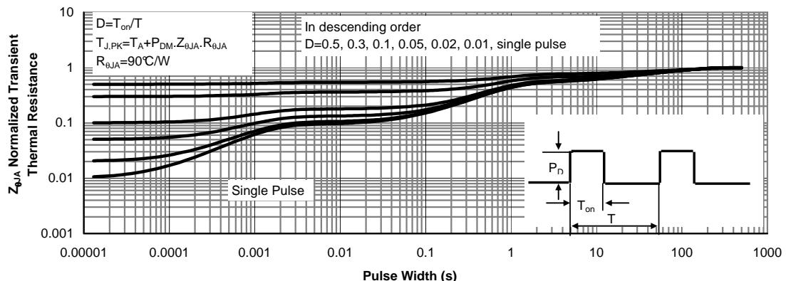
Figure 12: Normalized Maximum Transient Thermal Impedance (Note F)
