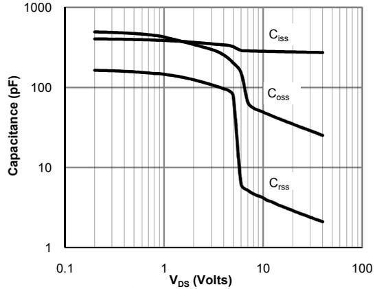
Figure 8: Capacitance Characteristics
