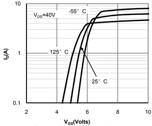
**Figure 2: Transfer Characteristics**
