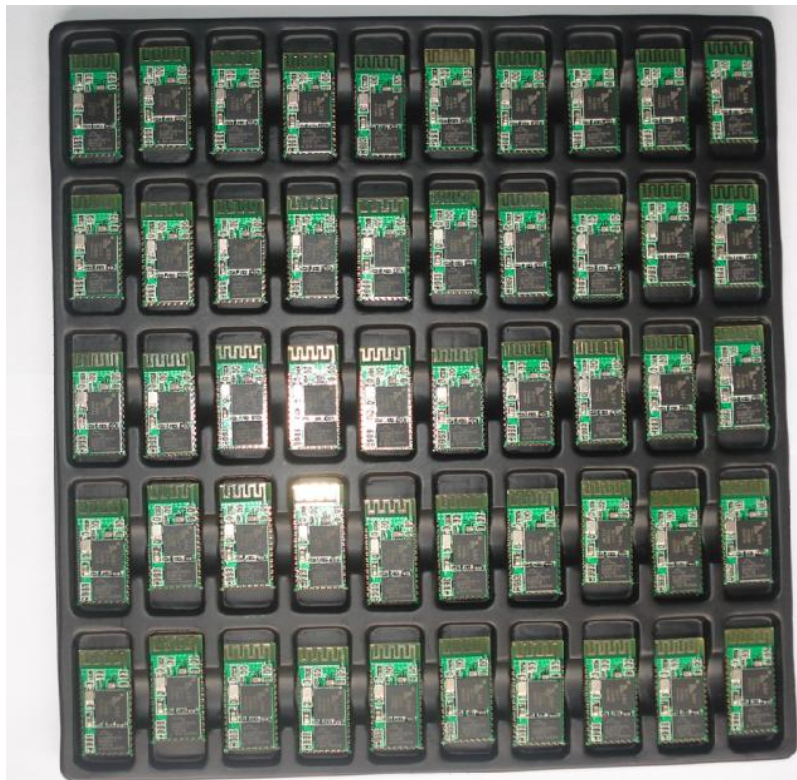
Figure 3 50 pieces chips in an anti-static blister package.
