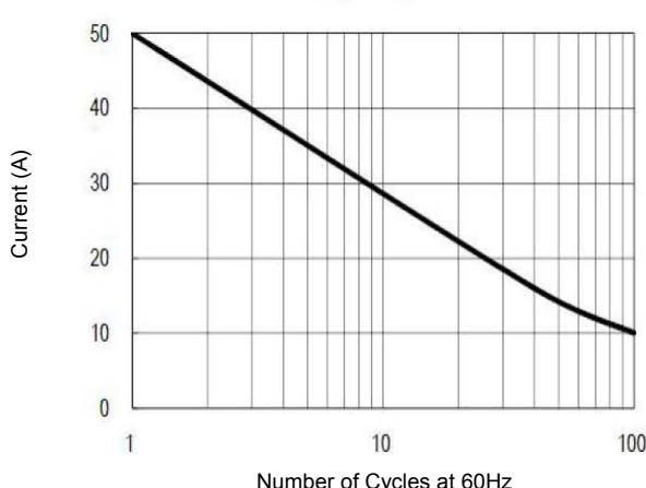
Figure 3. Maximum Non-Repetitive Forward Surge Current
