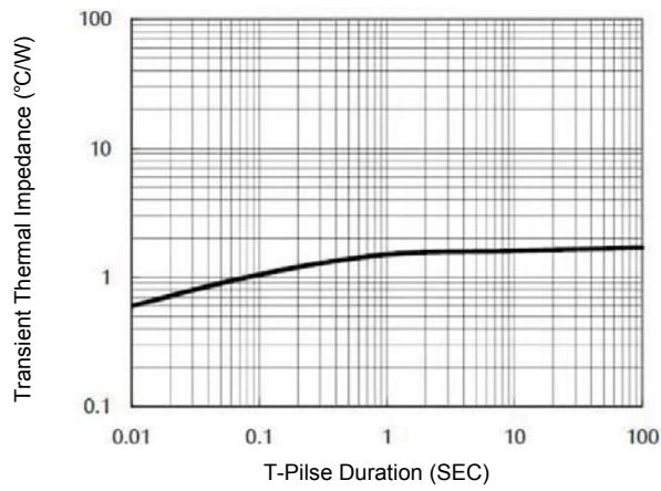
Figure 5. Typical Transient Thermal Characteristics
