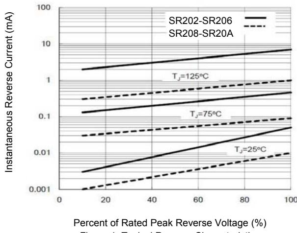
Figure 1. Typical Reverse Characteristics
