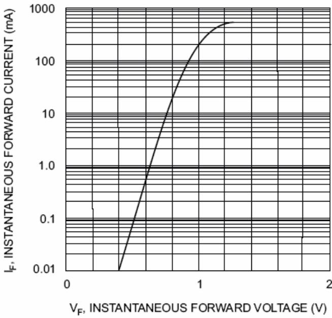
Fig. 1 Forward Characteristics
