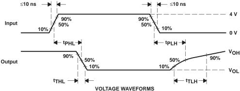
NOTES: A. The pulse generator has the following characteristics:  $Z_{O}$  = 50  $\Omega$ ,  $t_{W}$  = 500 ns.
