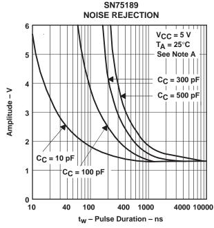
NOTE A: Maximum amplitude of a positive-going pulse that, starting from 0 V, will not cause a change in the output level.
