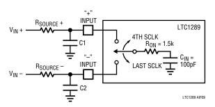
Figure 9. Analog Input Equivalent Circuit
