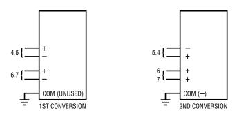
Figure 1. Examples of Multiplexer Options on the LTC1289
