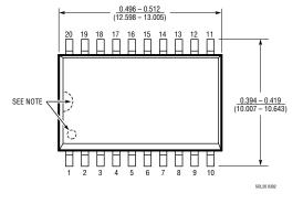
**NOTE:**PIN 1 IDENT, NOTCH ON TOP AND CAVITIES ON THE BOTTOM OF PACKAGES ARE THE MANUFACTURING OPTIONS. THE PART MAY BE SUPPLIED WITH OR WITHOUT ANY OF THE OPTIONS.
