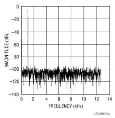
Figure 17a.  $f_{IN} = 1kHz$ ,  $f_{S} = 25kHz$ , SNR = 72.92dB
