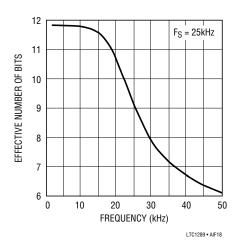
Figure 18. LTC1289 ENOB vs Input Frequency
