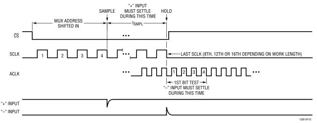
Figure 10. "+" and "-" Input Settling Windows
