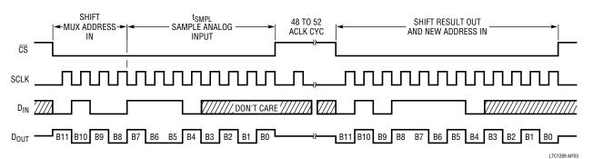
Figure 3. CS High During Conversion
