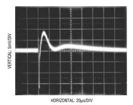
Figure 12. Poor Op Amp Settling Can Cause A/D Errors
