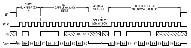
Figure 4. CS Low During Conversion
