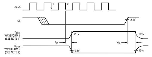
NOTE 1: WAVEFORM 1 IS FOR AN OUTPUT WITH CONDITIONS SUCH THAT THE OUTPUT IS HIGH UNLESS DISABLED BY THE OUTPUT CONTROL.
