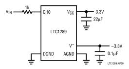
Figure 20. Overvoltage Protection for MUX
