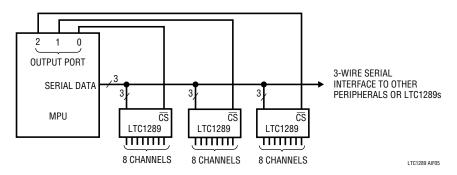
Figure 5. Several LTC1289s Sharing One 3-Wire Serial Interface
