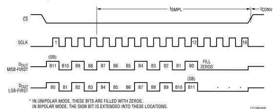
Figure 2. Data Output (D<sub>OUT</sub>) Timing with Different Word Lengths
