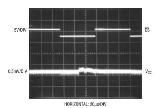
Figure 8b. Lithium Battery with 10µF Bypassing on V<sub>CC</sub>
