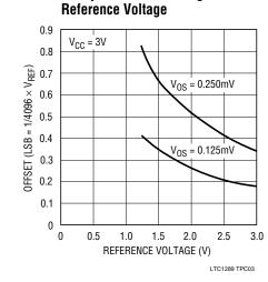
Unadjusted Offset Voltage vs
