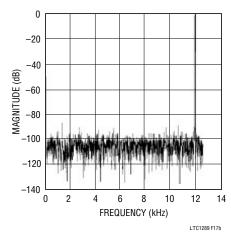
Figure 17b.  $f_{IN} = 12kHz$ ,  $f_{S} = 25kHz$ , SNR = 72.23dB
