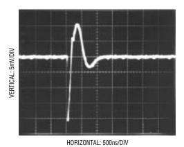
Figure 11. Adequate Settling of Op Amps Driving Analog Input
