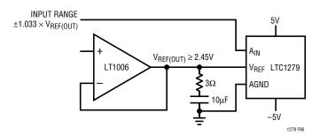
Figure 6. Driving the V<sub>REF</sub> with the LT1006 Op Amp
