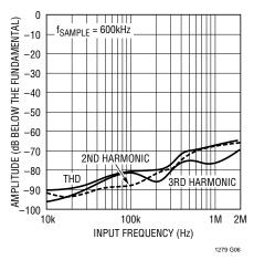
Figure 4. Distortion vs Input Frequency
