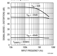
Signal-to-Noise Ratio (Without Harmonics) vs Input Frequency
