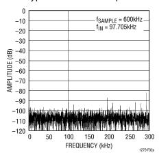
Figure 2a. LTC1279 Nonaveraged, 4096 Point FFT Plot with 100kHz Input Frequency
