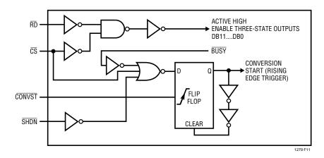
Figure 11. Internal Logic for Control Inputs CS, RD, CONVST and SHDN
