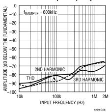
Peak Harmonic or Spurious Noise vs Input Frequency
