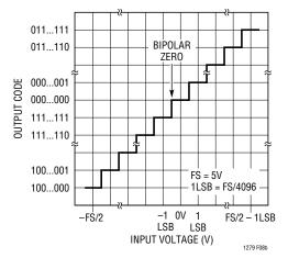
Figure 8b. LTC1279 Bipolar Transfer Characteristics
