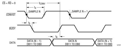
Figure 12. Mode 1a. CONVST Starts a Conversion. Data Ouputs Always Enabled. (CONVST = + )
