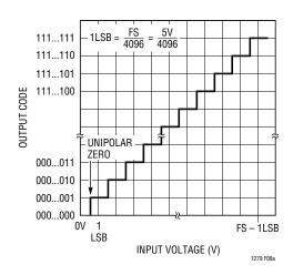
Figure 8a. LTC1279 Unipolar Transfer Characteristics
