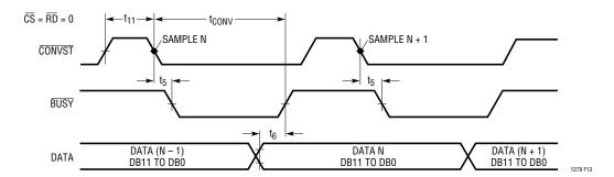
Figure 13. Mode 1b.  $\overline{\text{CONVST}}$  Starts a Conversion. Data Outputs Always Enabled. ( $\overline{\text{CONVST}} = \boxed{\uparrow}$
