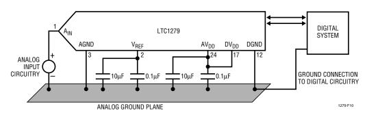
Figure 10. Power Supply Grounding Practice
