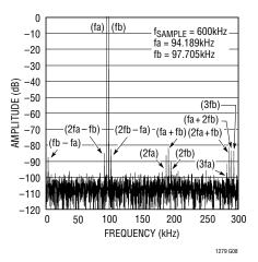
Figure 5. Intermodulation Distortion Plot
