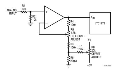
Figure 9c. LTC1279 Bipolar Offset and Full-Scale Adjust Circuit
