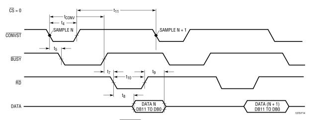
Figure 14. Mode 2.  $\overline{\text{CONVST}}$  Starts a Conversion. Data is Read by  $\overline{\text{RD}}$
