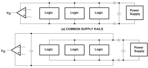
(b) SEPARATE BYPASSED SUPPLY RAILS (preferred)
