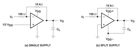
Figure 3. Gain-of-100 Inverting Amplifier
