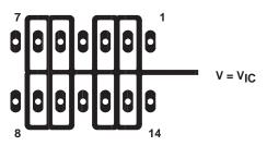
Figure 4. Isolation Metal Around Device Inputs (J and N packages)
