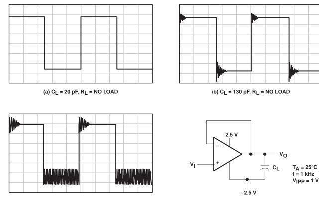
(c)  $C_L = 150 \text{ pF}$ ,  $R_L = \text{NO LOAD}$
