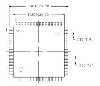
DIMENSIONS IN MILLIMETERS LEAD COPLANARITY 0.102 MAX.
