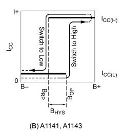
Figure 1. Alternative switching behaviors are available in the A114x device family. On the horizontal axis, the B+ direction indicates increasing south polarity magnetic field strength, and the B– direction indicates decreasing south polarity field strength (including the case of increasing north polarity).
