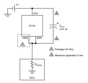
Figure 3. Typical application circuit
