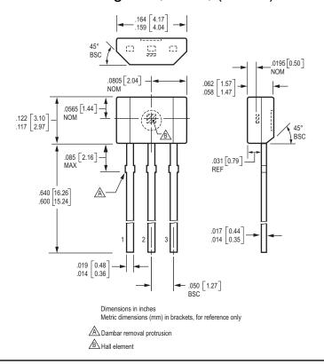
Sensitive Two-Wire Chopper-Stabilized Unipolar Hall Effect Switches
