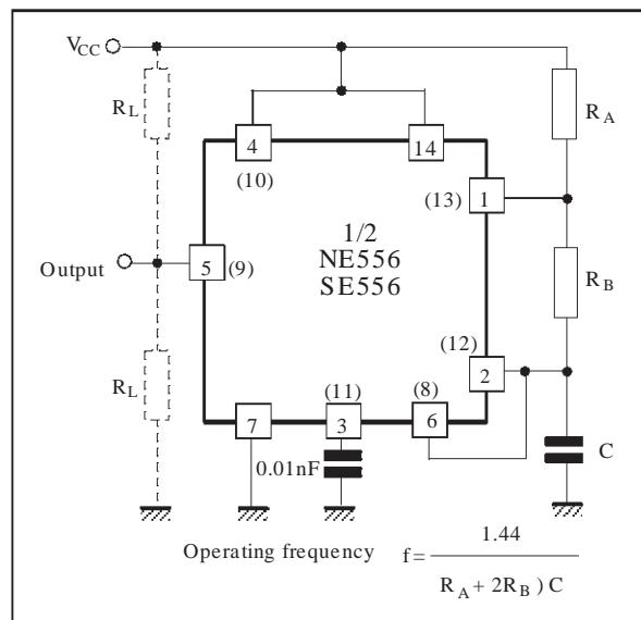
$$t_1 = 0.693 (R_A + R_B) C \text{ Output High}$$
