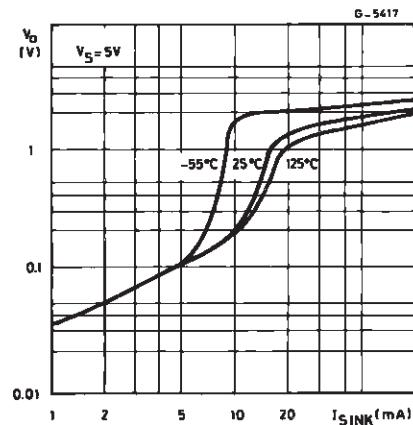
**Figure 5 :** Low Output Voltage versus Output Sink Current
