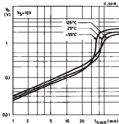
**Figure 6 :** Low Output Voltage versus Output Sink Current
