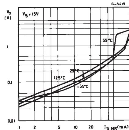
**Figure 7 :** High Output Voltage Drop versus Output
