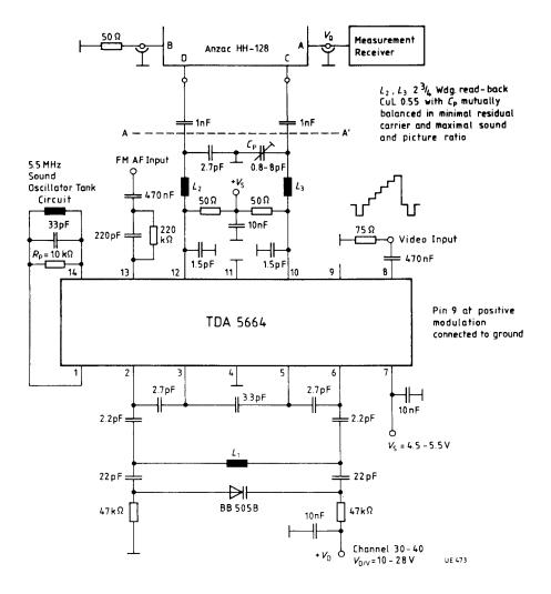
**Test Circuit 2** Measuring of the Modulation Depth for Positive and Negative Modulation
