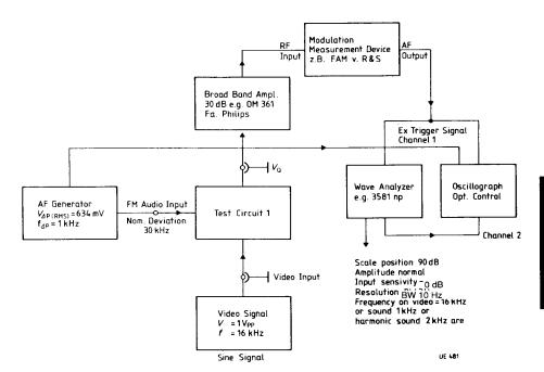
Calibration: AF signals are switched off, video signal is present at video input, modulation measurement device set at AM is adjusted to video carrier; filter: 300 Hz ... 20 kHz; detector: (P + P)/2; wave analyzer at video signal level (16 kHz) adjusted and resultant level as reference av defined.
