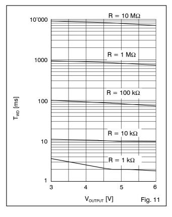
$T_{WD}$  versus R at  $T_J = +85\ ^{\circ}\text{C}$
