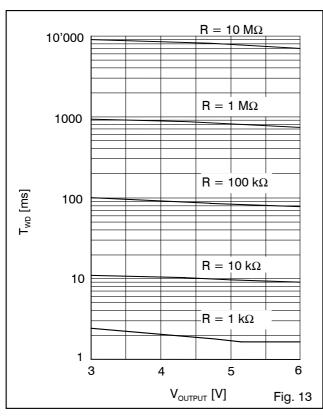
$T_{WD}$  versus R at  $T_J =$  -40 °C
