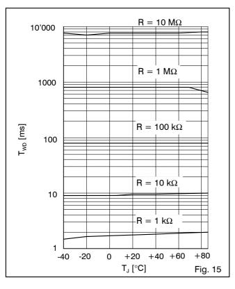
$T_{\,\text{WD}}$  versus R at 5 V
