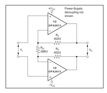
Figure 5. Noninverting Differential I/O Amplifier
