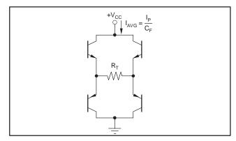
Figure 9. Output Stage Power Model
