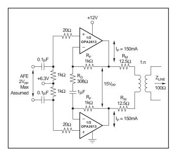
Figure 6. Single-Supply ADSL Upstream Driver
