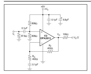
Figure 3. AC-Coupled, G = +2, Single-Supply, Specification and Test Circuit
