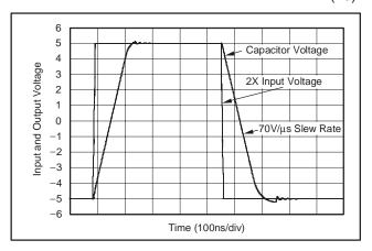
Figure 12. Large-Signal Capacitive Load Drive
