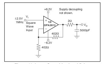
Figure 11. Large Capacitive Load Driver
