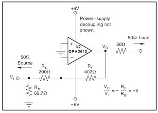
Figure 10. Inverting Gain of -1 with Impedance Matching
