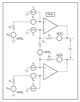
Figure 14. Differential Op Amp Noise Analysis
