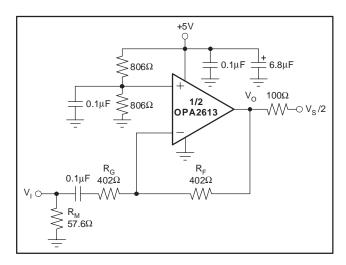
Figure 4. AC-Coupled, G = -1, Single-Supply, Specification and Test Circuit
