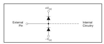
Figure 15. Internal ESD Protection
