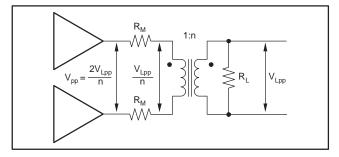
Figure 7. Driver Peak Output Voltage
