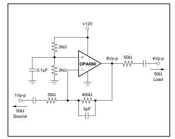
FIGURE 6. High Power Coax Line Driver.
