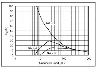
FIGURE 10. Required R<sub>s</sub> vs Noise Gain.
