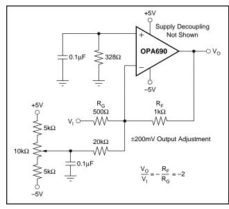
FIGURE 12. DC-Coupled, Inverting Gain of –2, with Offset Adjustment.
