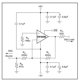
FIGURE 8. Gain of -2 Example Circuit.
