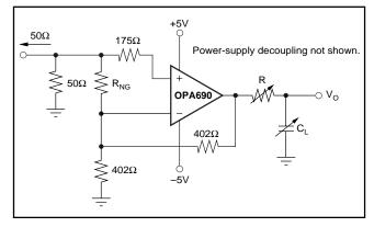
FIGURE 9. Capacitive Load Driving with Noise Gain Tuning.
