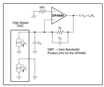
FIGURE 5. DAC Transimpedance Amplifier.
