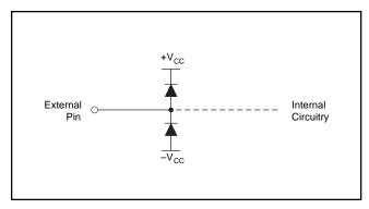
FIGURE 15. Internal ESD Protection.
