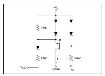
FIGURE 13. Simplified Disable Control Circuit.
