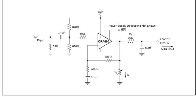
FIGURE 3. Single-Supply ADC Input Driver.
