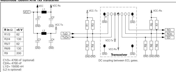
The power supply filtering is required for good EMI performance. Use short tracks from the inductor L1/L2 to the module  $V_{CC}$ -Rx/ $V_{CC}$ -Tx.
