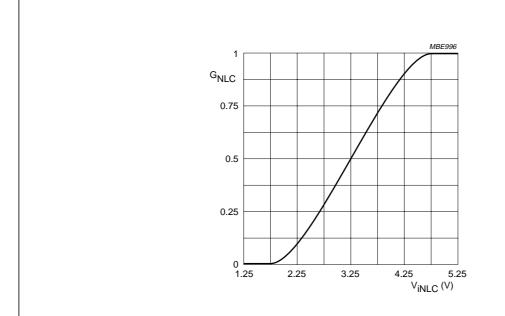
Fig.5 Non-linear amplifier gain as a function of input voltage at pin NLC.
