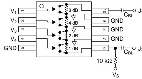
DC blocking capacitors ( $C_{BL}$ ) and biasing resistor must be supplied externally for positive voltage operation.
