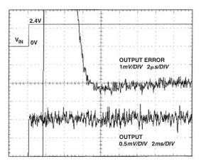
Figure 12. Turn-On Settling
