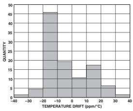
Figure 1. Reverse Voltage Temperature Drift Distribution
