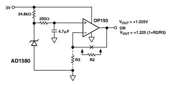
Figure 15. Micropower Buffered Reference
