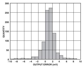
Figure 2. Reverse Voltage Error Distribution
