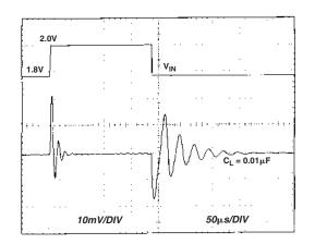
Figure 14. Transient Response with Capacitive Load
