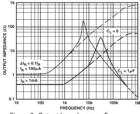
Figure 8. Output Impedance vs. Frequency
