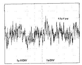
Figure 9. 0.1 Hz to 10 Hz Voltage Noise
