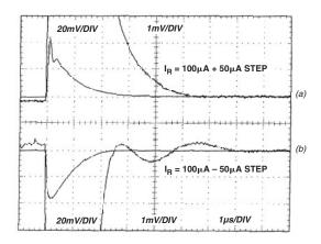
Figure 13. Transient Settling
