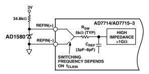
Figure 16. Reference Circuit for the AD7714/AD7715-3
