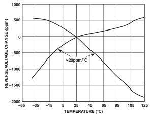
*TPC 1. Output Drift for Different Temperature Characteristics*
