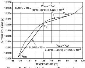
Figure 5. Output Voltage vs. Temperature
