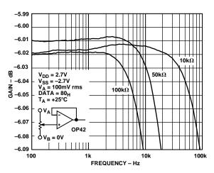
Figure 5. Gain Flatness vs. Frequency
