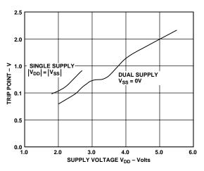
Figure 11. Digital Input Trip Point vs. Supply Voltage
