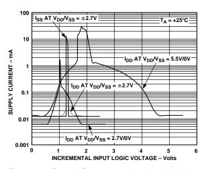
Figure 12. Supply Current vs. Input Logic Voltage
