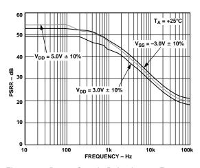
Figure 14. Power Supply Rejection vs. Frequency
