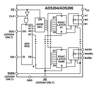
Figure 17. Block Diagram
