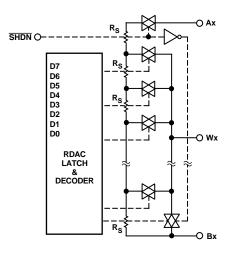
Figure 16. AD5204/AD5206 Equivalent RDAC Circuit
