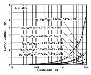
Figure 13. Supply Current vs. Clock Frequency
