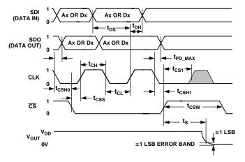
Figure 2. Detail Timing Diagram
