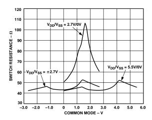
Figure 4. Incremental Wiper ON Resistance vs. Voltage
