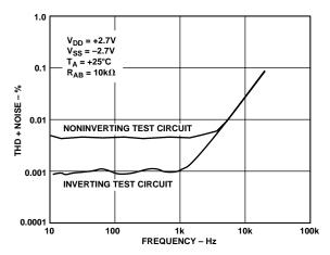
Figure 15. Total Harmonic Distortion Plus Noise vs. Frequency
