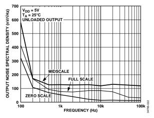
Figure 22. Noise Spectral Density
