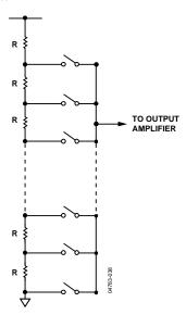
Figure 39. Resistor String Structure
