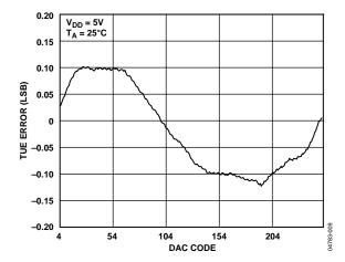
Figure 9. AD5601 Total Unadjusted Error (TUE)
