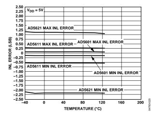
Figure 25. INL vs. Temperature (5 V)
