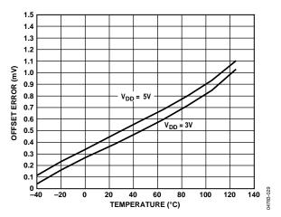
Figure 29. Offset Error vs. Temperature (5 V)
