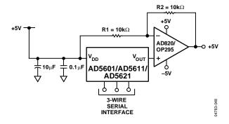
Figure 51. Bipolar Operation with the AD5601/AD5611/AD5621
