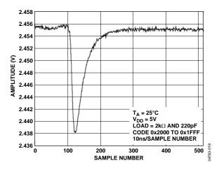
Figure 18. Digital-to-Analog Glitch Energy
