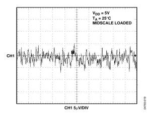
Figure 19. 1/f Noise, 0.1 Hz to 10 Hz Bandwidth
