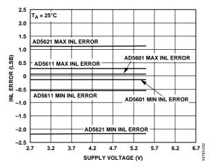
Figure 32. INL vs. Supply Voltage at 25°C
