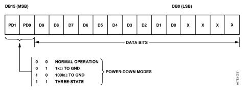
Figure 41. AD5611 Input Register Contents
