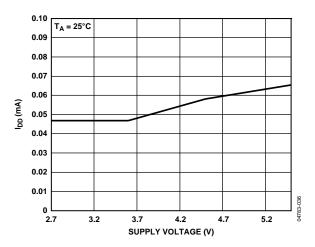
Figure 36. Supply Current vs. Supply Voltage at 25°C
