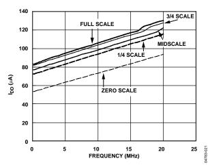
Figure 21. IDD vs. SCLK vs. Code
