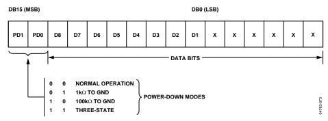
Figure 42. AD5601 Input Register Contents
