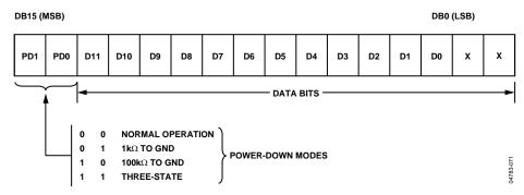
Figure 40. AD5621 Input Register Contents
