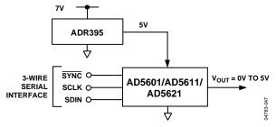
Figure 50. ADR395 as Power Supply to the AD5601/AD5611/AD5621
