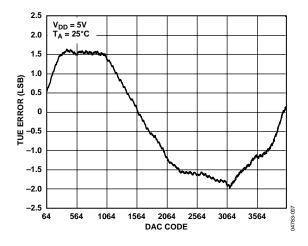
Figure 7. AD5621 Total Unadjusted Error (TUE)
