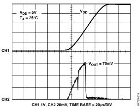
Figure 16. Power-On Reset to 0 V
