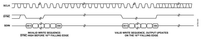
Figure 43. SYNC Interrupt Facility
