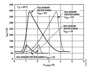
Figure 37. SCLK/SDIN vs. Logic Voltage
