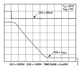
Figure 14. Full-Scale Settling Time
