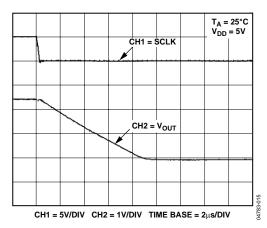
Figure 15. Half-Scale Settling Time
