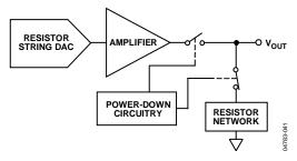
Figure 44. Output Stage during Power-Down
