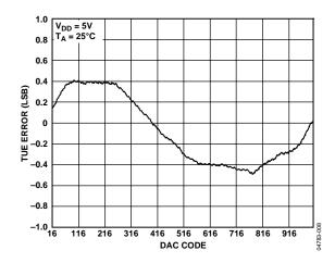
Figure 8. AD5611 Total Unadjusted Error (TUE)
