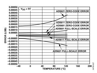
Figure 27. Zero-Code and Full-Scale Error vs. Temperature
