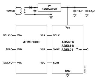
Figure 52. AD5601/AD5611/AD5621 with a Galvanically Isolated Interface
