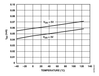
Figure 31. Supply Current vs. Temperature (5 V)
