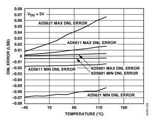
Figure 26. DNL vs. Temperature (5 V)
