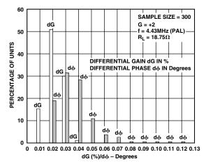
Figure 3. Distribution of Differential Gain (dG) and Differential Phase ( $d\phi$ );  $R_L$  = 18.75  $\Omega$
