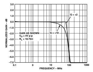
Figure 20. Large Signal Frequency Response;  $V_0 = 4 V p-p$
