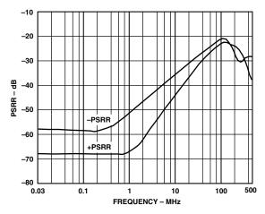
Figure 15. PSRR vs. Frequency
