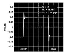
Figure 21. Small-Signal Pulse Response; G = +1
