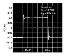
Figure 22. Small-Signal Pulse Response; G = +2, -1
