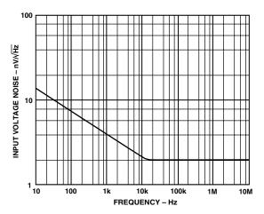
Figure 23. Input Voltage Noise vs. Frequency
