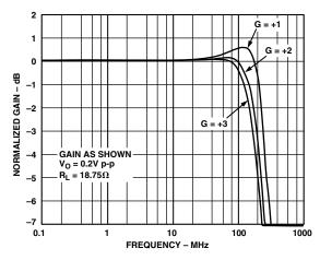
Figure 11. Small Signal Closed-Loop Frequency Response;  $R_L$  = 18.75  $\Omega$
