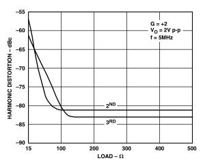
Figure 13. Harmonic Distortion vs. Load
