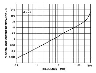
Figure 16. Closed-Loop Output Resistance vs. Frequency
