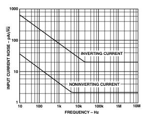
Figure 26. Input Current Noise vs. Frequency
