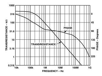
Figure 19. Transresistance and Phase vs. Frequency;  $R_L=18.75\,\Omega$
