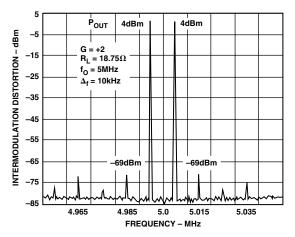
Figure 9. Intermodulation Distortion
