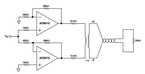
Figure 31. High Output Differential Line Driver Using Two AD8010s. NOTE: Please see Figure 29 for Recommended Bypassing Technique.
