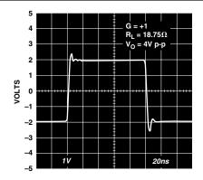
Figure 24. Large-Signal Pulse Response; G = +1
