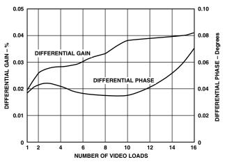
Figure 6. Differential Gain and Phase vs. Number of Video Loads Over Temperature (–40°C to +85°C); f = 4.43 MHz
