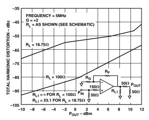
Figure 10. Total Harmonic Distortion vs.  $P_{OUT}$ ; G = +2
