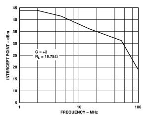
Figure 7. Two-Tone, 3rd Order IMD Intercept vs. Frequency; G = +2,  $R_L = 18.75 \Omega$
