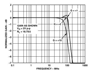
Figure 17. Large Signal Frequency Response;  $V_0 = 2 V p-p$
