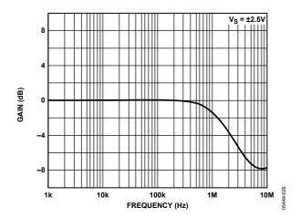
Figure 25. Output Buffer Gain vs. Frequency
