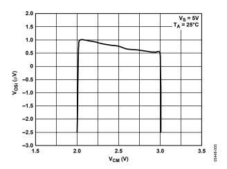
Figure 5. Input Offset Voltage vs. Common-Mode Voltage
