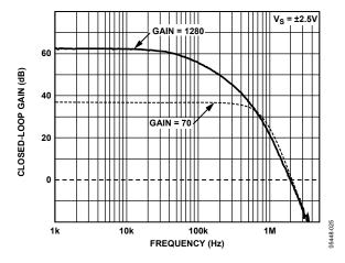
Figure 24. Closed-Loop Gain vs. Frequency Measured at Output Pin
