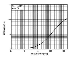
Figure 39. Output Impedance vs. Frequency
