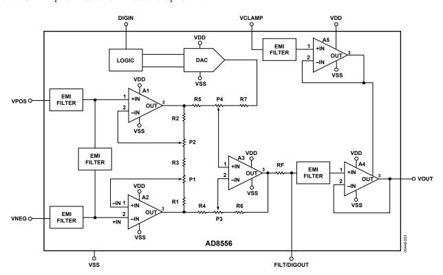
Figure 51. Block Diagram Showing EMI/RFI Built-In Filters
