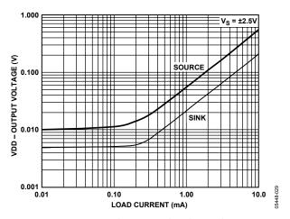
Figure 28. Output Voltage to Supply Rail vs. Load Current
