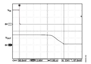
Figure 41. Positive Overload Recovery (Gain = 70)
