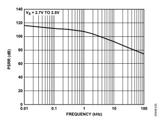
Figure 34. PSRR vs. Frequency
