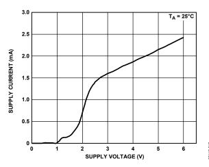
Figure 14. Supply Current (Isy) vs. Supply Voltage
