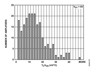
Figure 7.  $T_cV_{OS}$  at  $V_{SY} = 5 V$
