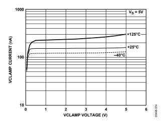
Figure 13. VCLAMP Current over Temperature at  $V_5 = 5 \text{ V vs. VCLAMP Voltage}$
