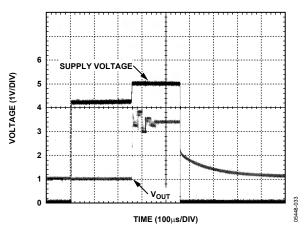
Figure 32. Power-On Response at −40°C
