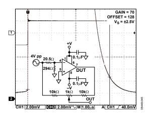
Figure 44. Settling Time 0.1%
