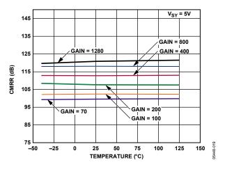
Figure 18. CMRR vs. Temperature at Different Gains
