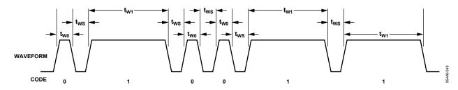
Figure 49. Timing Diagram for Code 010011
