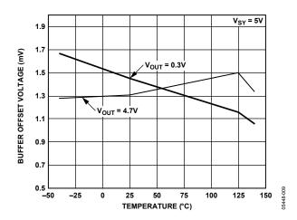
Figure 8. Output Buffer Offset vs. Temperature
