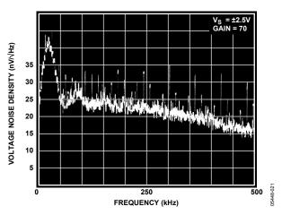
Figure 20. Input Voltage Noise Density vs. Frequency (0 Hz to 500 kHz)
