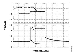
Figure 30. Power-On Response at 25°C
