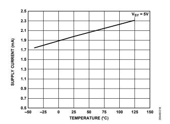
Figure 15. Supply Current (I<sub>SY</sub>) vs. Temperature
