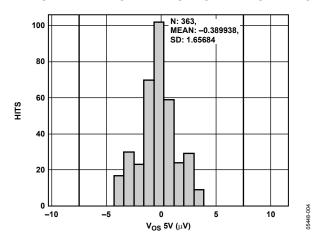
Figure 4. Input Offset Voltage Distribution
