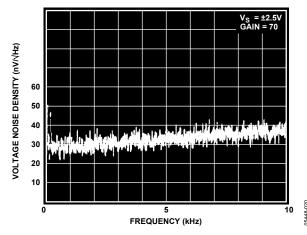
Figure 19. Input Voltage Noise Density vs. Frequency (0 Hz to 10 kHz)
