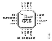
Figure 3.16-Lead LFCSP\_VQ Pin Configuration
