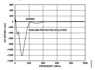
Figure 55. Response of AD8556 to EMI/RFI Differential Signals
