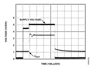
Figure 31. Power-On Response at 125°C
