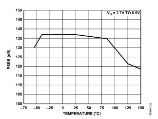
Figure 33. PSRR vs. Temperature
