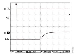
Figure 42. Negative Overload Recovery (Gain = 1280)
