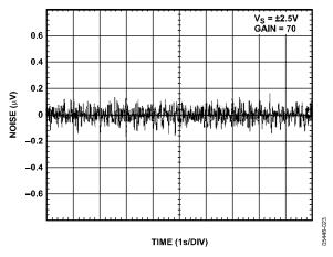
Figure 22. Low Frequency Input Voltage Noise (0.1 Hz to 10 Hz)
