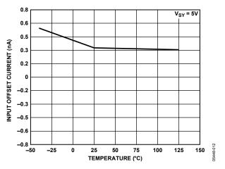
Figure 11. Input Offset Current vs. Temperature
