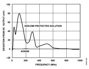
Figure 53. DC Offset Values at V<sub>OUT</sub> Caused by Frequency Seep of Input
