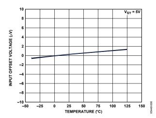
Figure 6. Input Offset Voltage vs. Temperature
