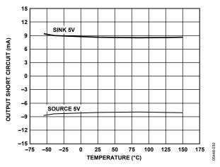
Figure 29. Output Short-Circuit vs. Temperature
