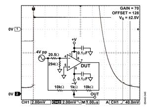
Figure 45. Settling Time 0.01%
